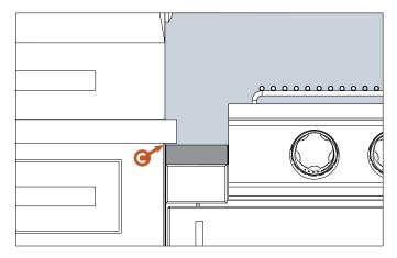
The countertop should be adhered directly to the tops of the cabinets using silicone adhesive. See detailed instructions in the cabinetry installation manual.
