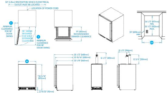
\*LEVELLING LEGS CAN ADD UP TO 3/4" (19mm) to HEIGHT
