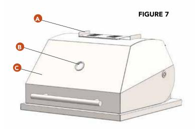
IMPORTANT: To avoid collecting excessive rain water, keep the lid vent closed when the grill is not in use.
