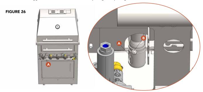
Loosen the screw that secured the air shutter (see Figure 26:B). Use care not to remove the screw by loosening too far. Adjust the air shutter until the flames burn blue, are stable, and do not lift off the burner. Secure the air shutter in position by re-tightening the screw.
