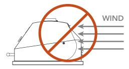
Optional stainless steel wind screens are available from Kalamazoo Outdoor Gourmet. If you are building your own wind break wall, we recommend a minimum height of 24 inches (610mm) above the countertop, and a minimum of 2 inches (51mm) wider than the base of the grill. These minimum dimensions are for a wall positioned 3.5 inches (89mm) from the back of the grill. The further behind the grill a wind wall is placed, the larger it needs to be.
