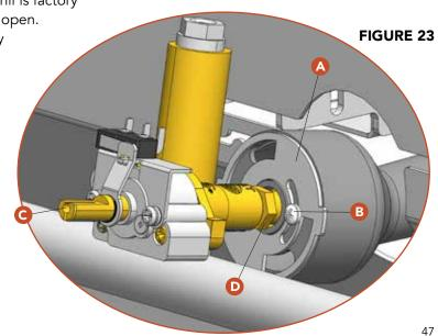
Reinstall the burner into the grill, being careful to ensure the burner is seated properly over the orifice (Figures 20:E and 23:D) and the locating posts (Figure 20:F) are seated into the burner support brackets. Test the burner on HIGH for proper flame characteristics before reinstalling the burner guard.
