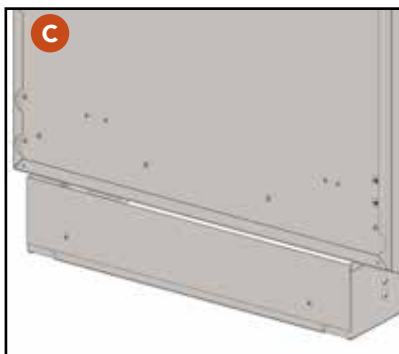
SIDE TOE KICKS CONNECT TO FRONT AND REAR TOE KICKS, OR TO FRONT TOE KICK AND REAR LEG
