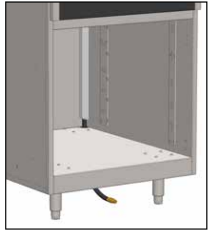
REPLACE GAS LINE COVER. SECURE WITH SCREW AT TOP
