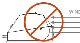
Do not place the grill in a location where the rear hood openings are likely to be exposed to strong wind. A wind break wall is recommended for installations where the prevailing wind may be a problem.
