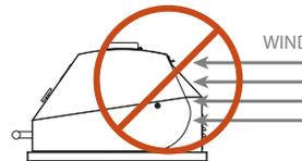
Do not place the grill in a location where the rear hood openings are likely to be exposed to strong wind. A wind break wall is recommended for installations where the prevailing wind may be a problem.
