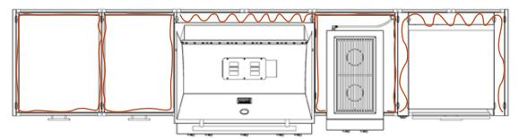
A SILICONE BEAD AROUND THE TOP OF EACH CABINET SECURES THE COUNTERTOP
