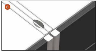
**9.** The bottoms of adjacent cabinets connect together with clips that secure with the included thumb screws.
