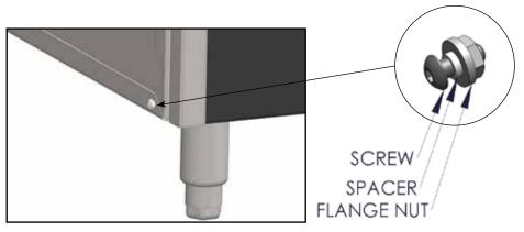
INSTALL THE SCREWS, SPACERS AND NUTS FOR MOUNTING THE END FINISHING PANELS
