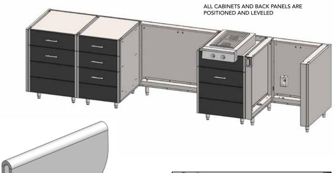
7. The tops of each cabinet and filler panel connect to adjacent units at the tops using the included Kalamazoo Speed Clips. These clips make installation easier. The unique design allows you to use the "ears" to draw together two units and ensure a snug fit.
