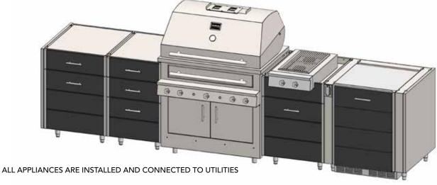
**14.** Install the front and back toe kicks by clipping them on to the cabinet legs. Toe kicks are adjustable in height. Loosen the screws slightly to slide the rear layer upward to contact then bottom of the cabinet. Then re-tighten the screws.
